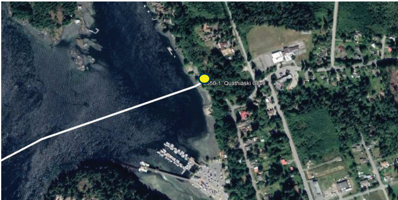
Connected Coast submarine fibre landing site at Quathiaski Cove. There is no proposed terrestrial fibre. White = Submarine fibre
