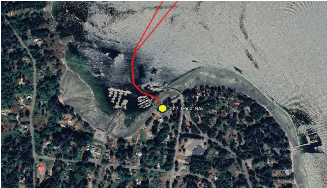
Connected Coast submarine fibre landing site at Heriot Bay. There is no propose terrestrial fibre. Red = Submarine fibre
