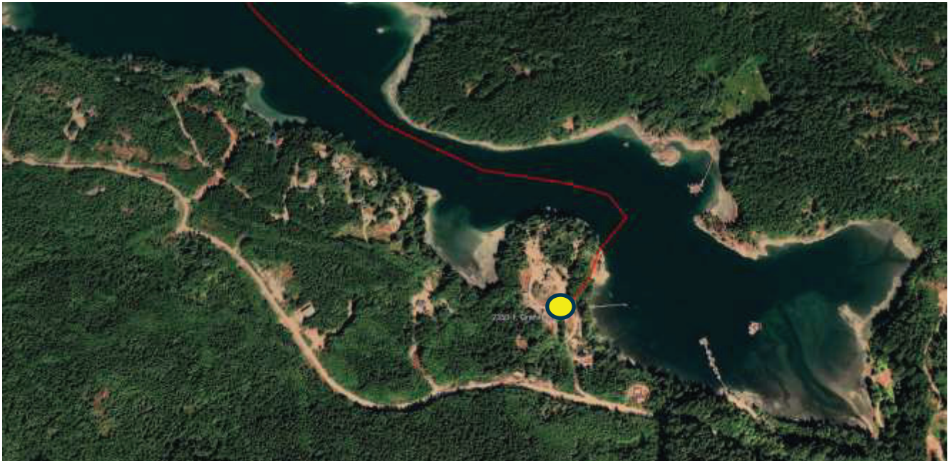
Connected Coast submarine fibre landing site at Granite Bay. There is no proposed terrestrial fibre. Red = Submarine fibre
