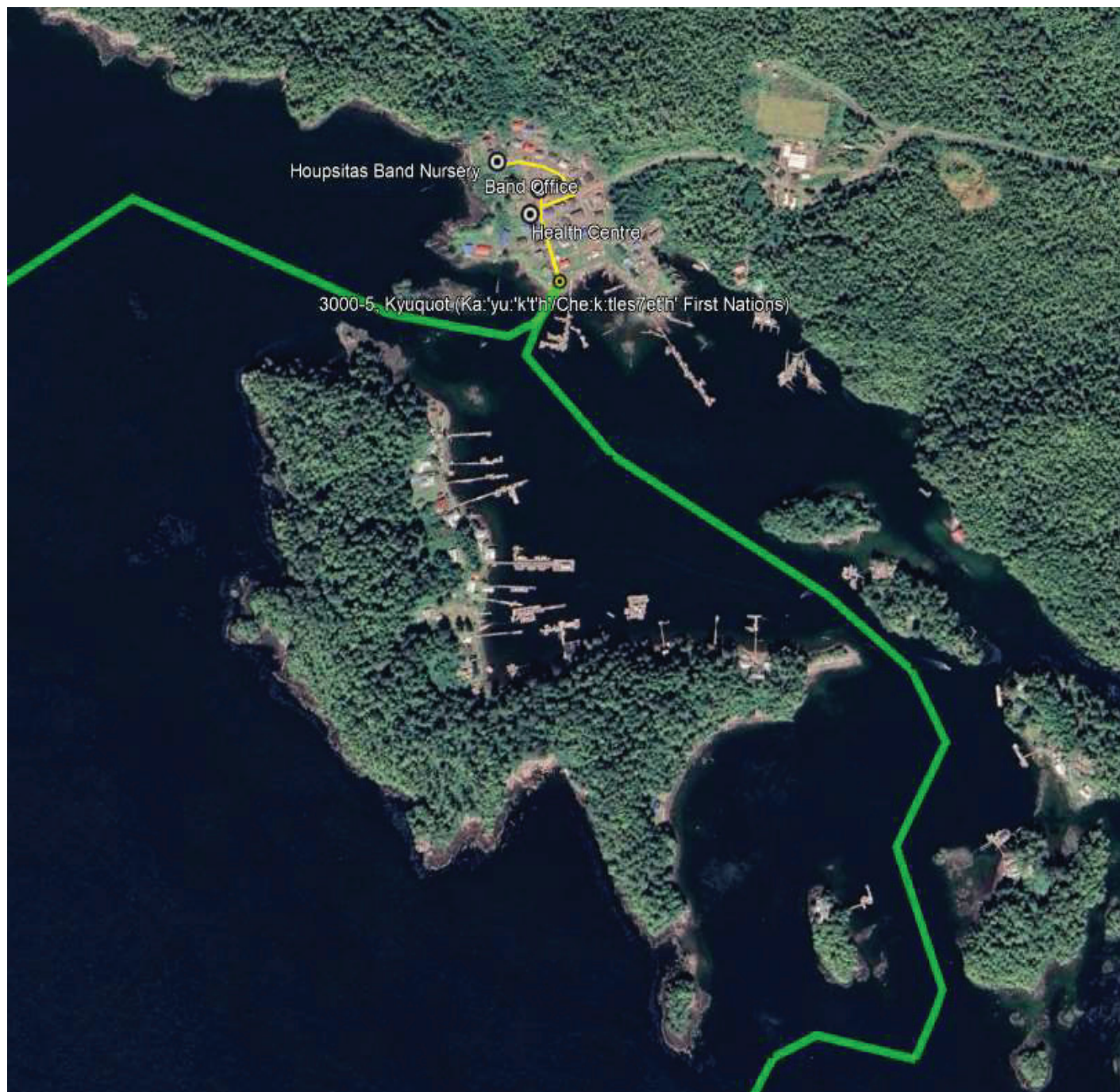
Connected Coast - Proposed backbone submarine fibre path and landing points (Estimated Completion 2021) Green = Main Submarine Fibre
