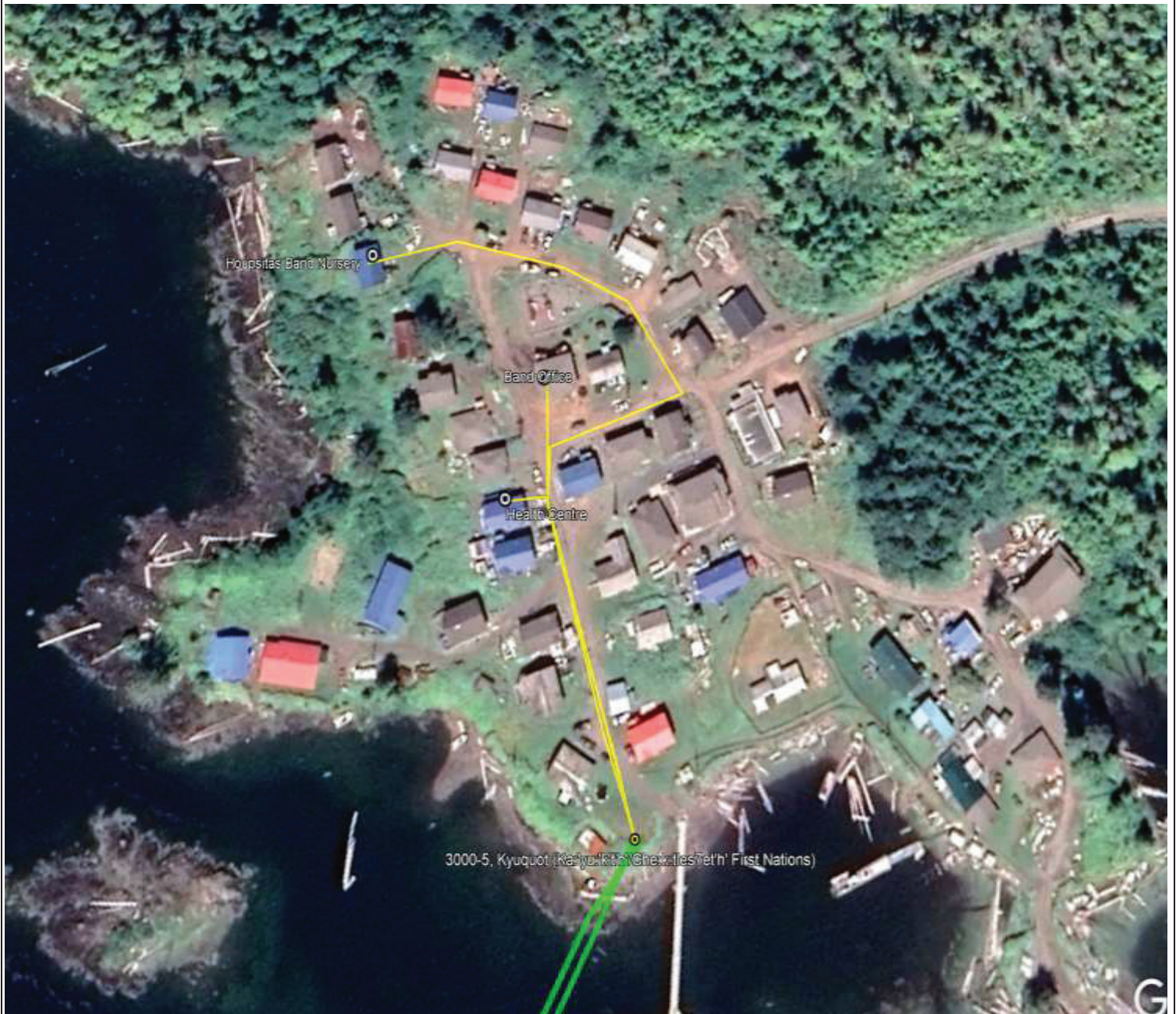
Connected Coast submarine fibre landing site at Kyuquot and terrestrial fibre build Green = Submarine Fibre Yellow Line = Terrestrial Fibre
