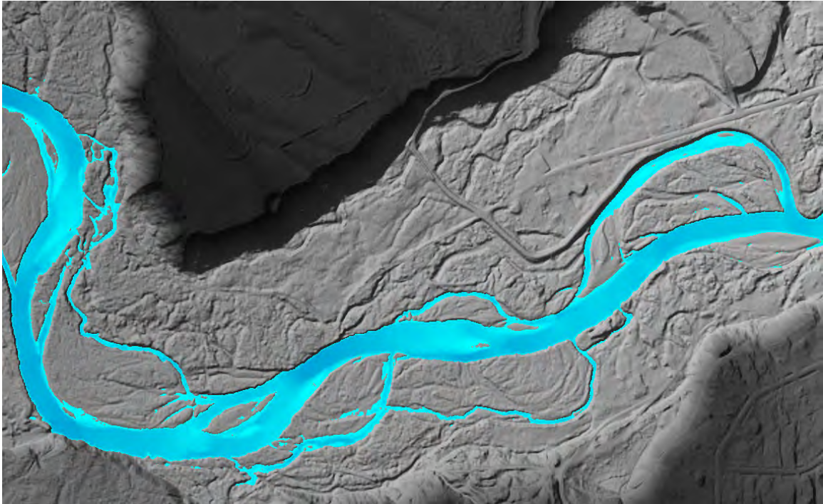
Figure 5: Digital Terrain Model (DTM) Shown in Grey Hillshade & Oyster River Main Flow Channels (Light Blue)
