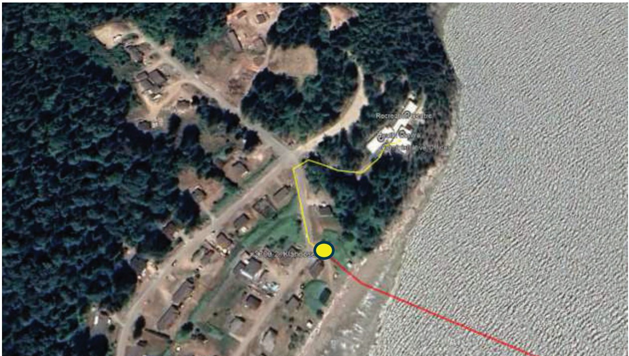
Connected Coast submarine fibre landing site at Klahoose First Nations. Red = Submarine fibre Yellow = Terrestrial fibre
