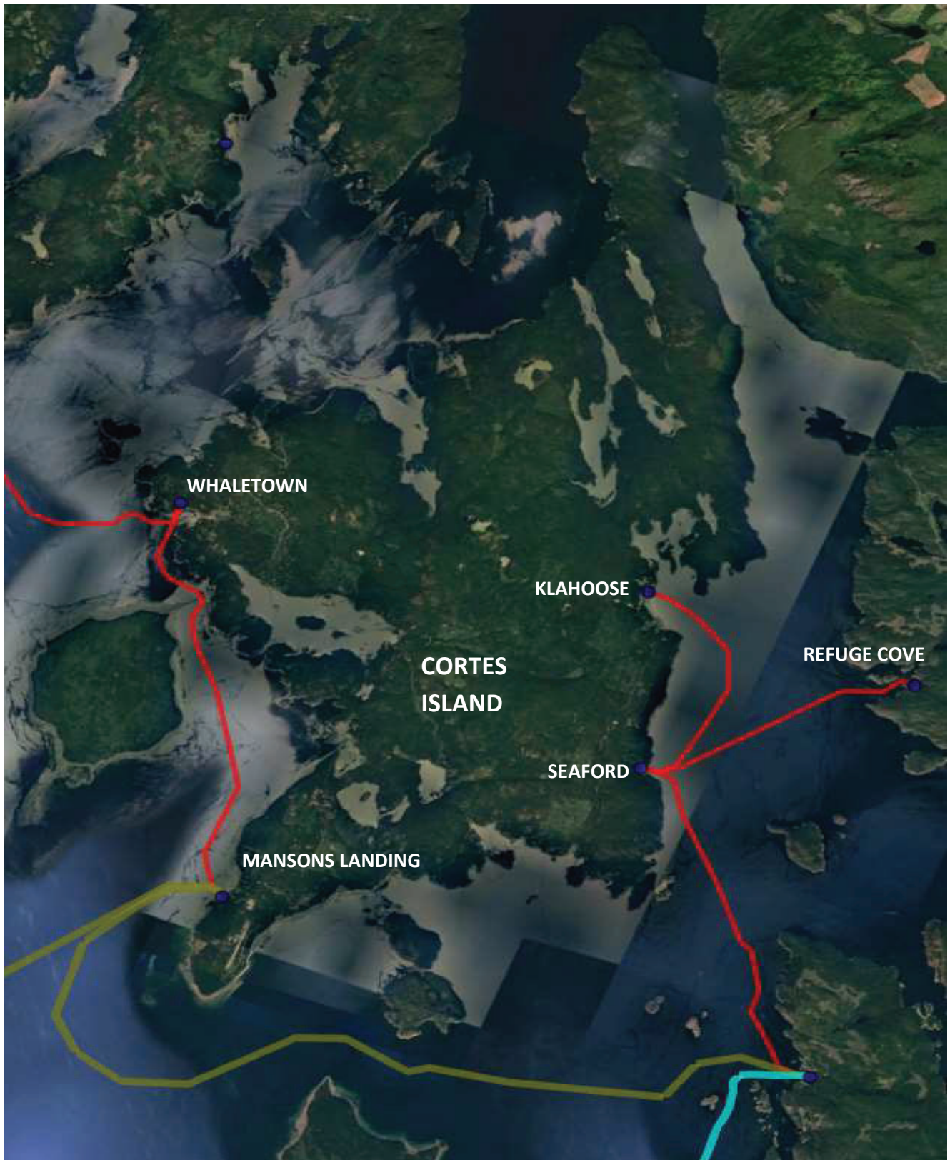
Connected Coast - Proposed backbone submarine fibre path and landing points (Estimated Completion 2021) Red, Blue & Green = Main submarine fibre
