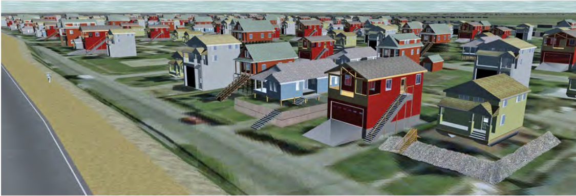
Figure 12: Examples of Raised Building Pads for Foundations 27
