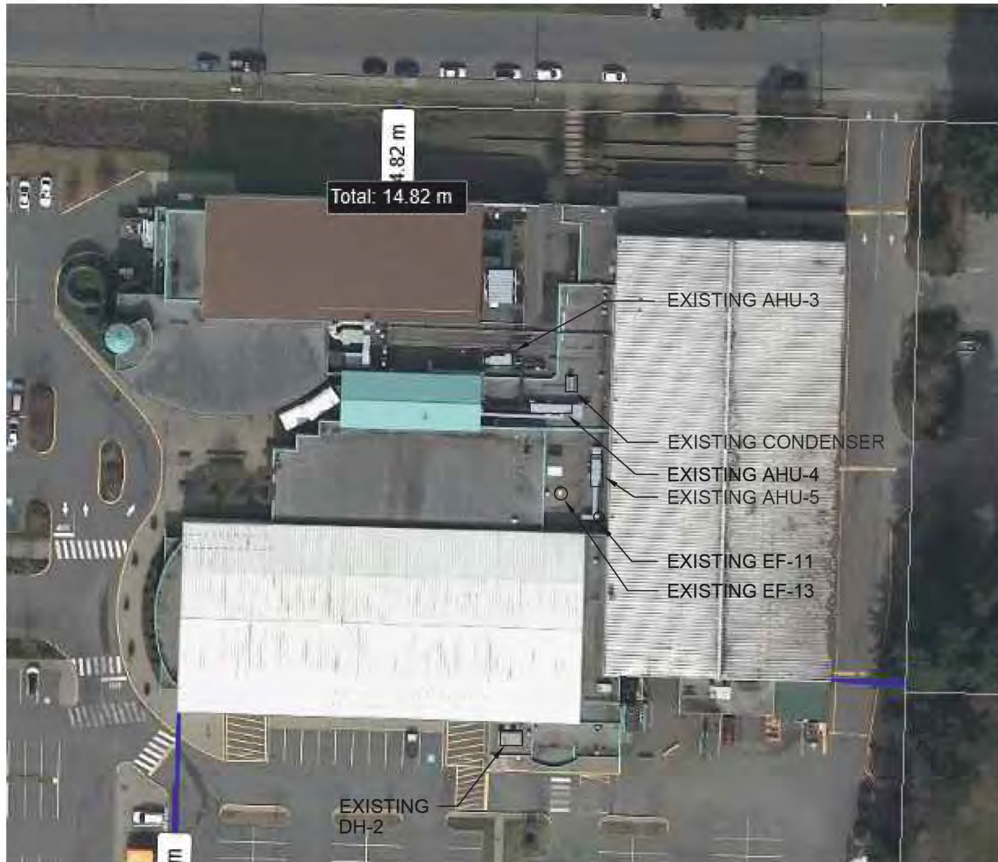
01 EXISTING ROOF/SITE PLAN M1 SCALE: NTS
